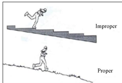
Fig. 11. Using ramps instead of stairs (National Building Regulations: Topic 21)
