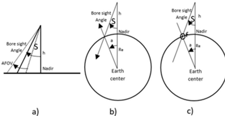
Fig. 1. Determining the satellite image coverage for three modes, flat Earth and spherical Earth (Feizi & Khazaei, 2017)
