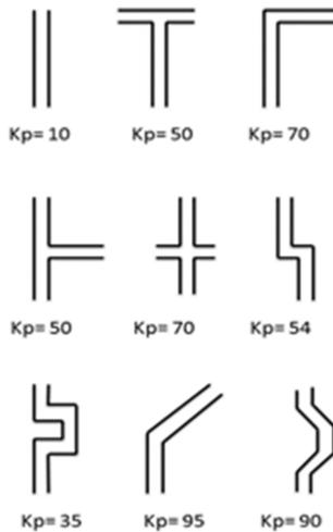
Fig. 5. Comparison between some of wave pressure reductive bends
